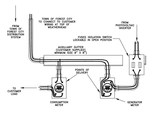
CONSUMPTION METER AND GENERATOR METER
